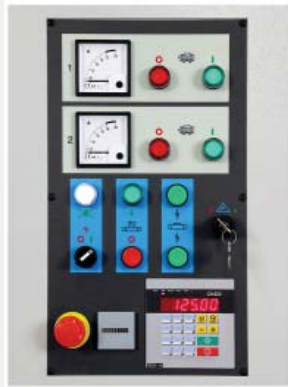
Control panel with digital thickness control, ammeters for each sanding head, and hour meter
