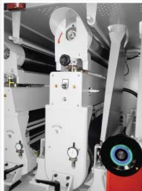
"D" Contact drum with optional air jet belt cleaning
