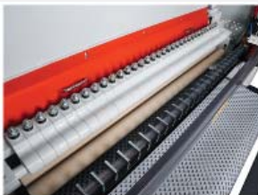
Sectional safety kickback fingers and sectional chipbreakers
