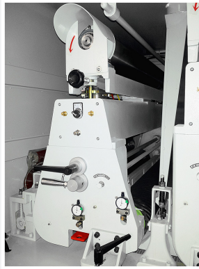
"A" combination sanding head with adjustable sanding pad
