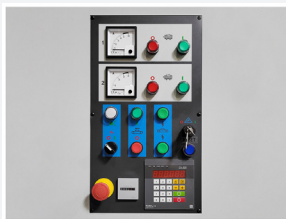
Control panel with digital thickness controller, individual ammeters for each sanding unit, and hour meter
