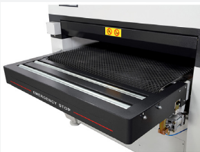
Infeed bed with rubber feed conveyor and conveyor belt tracking
