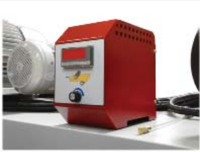
Inverter controlled variable planing speed
