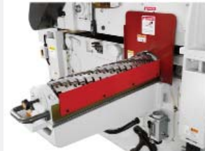
Removeable bottom spiral insert knife cutterhead
