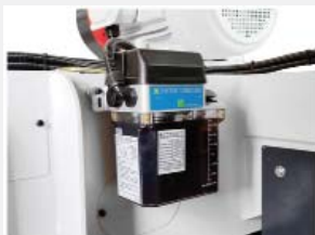
Auto lubrication to feed conveyor
