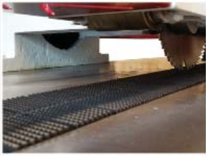
Precision machined cast iron chain and track assembly
