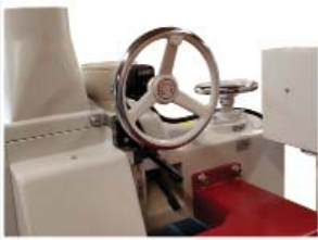
Pressure roller adjustment and blade height adjustment handwheel
