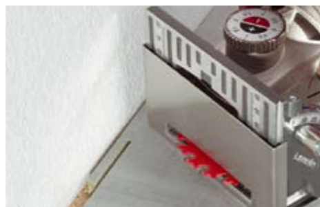
Cuts for expansion gaps (Saw blade Art.No. 132380 and sliding shoe Art.No. 251057)
