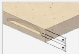
Adjust groove to middle
