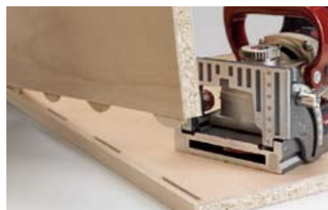
Joints with wood biscuits
