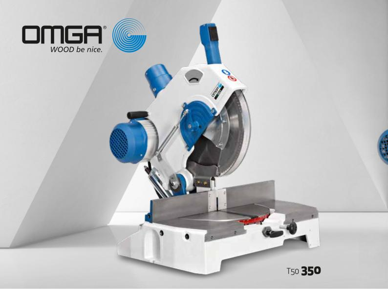
Precision mitre saws with rotating table and selfcentering locking for the main angles 90°, 45°, 30°, 22°,30′, 15°, 10° right and left; manual locking for all the other intermediate angles, with reading on the scale. The main characteristics of these mitre saws: structure in cast iron, motor of 2.2 kW with transmission by belt and blade of ø 350 mm. (ø 370 mm. on the model T 53), they ensure an absolute strength and a large cutting capacity.
