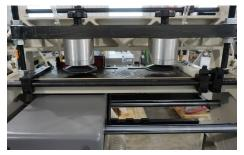
**CLAMPING SYSTEM.** Four pneumatic clamps hold materials firmly in place during operations. Clamps adjusted via individual lever activation.
