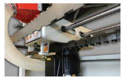
**MOTOR & TEMPLATES.** Four dovetail templates offer a range of dovetail joints using powerful 1HP spindle motor.
