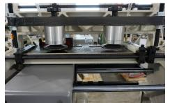
**CLAMPING SYSTEM.** Four pneumatic clamps hold materials firmly in place during operations. Clamps adjusted via individual lever activation.
