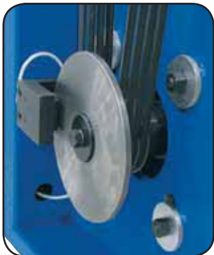
Pneumatic disk brakes to stop the working units within seconds from emergency.
