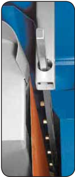
Separate dust hood for sanding belt cleaning blowers
