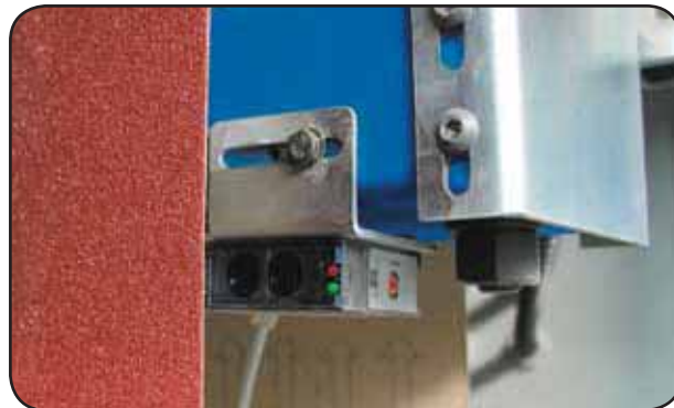
Sanding belt oscillation system with electronic dual-photocell. Safety micro-switch to stop the machine in case of breakage of the abrasive belt .
