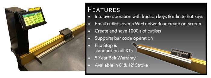
RazorGage XT offers amazing software functionality without breaking the bank including a Work Order screen that lets you create and save thousands of cutlists. Set up a free Gmail account to email cutlists to the machine (requires Wi-fi and internet access).
