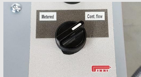
2-functions switch (1) Continuous glue flow, manual mode; (2) Metered glue dosing.
