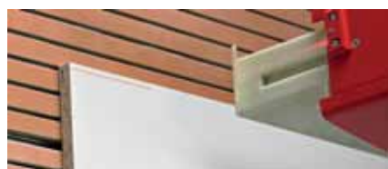
Laser-assisted indication of the horizontal cut (standard feature)
