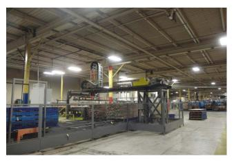
The MANYX destacker is an equipment that allows to feed lumber without operators in many types of woodworking equipment like moulder, planers or optimizing lines for examples. The MANYX can feed and separate layers of incoming lumber bundles, with or without sticks, random width and lengths or even some profiled boards depending on the final configuration.
