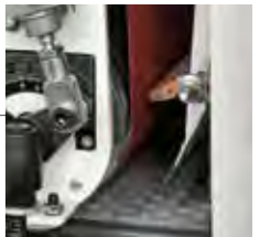
Exhaust hood for the dust dispersion control during processing
