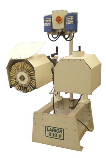
The LARICK 230 Series Profile Sander is a two spindle machine designed for use with flexible brush type sanding wheels. The spindles adjust individually, with vertical, horizontal, tilt and rotation. It can be placed at the outfeed end of a moulder, over a table, or used to sand free-hand.
