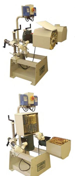
The spindles on the Larick Model 230 adjust individually to sand the top, bottom, front, or back of parts. In addition to the built in adjustment of the may stands. the stands slide forward/back on the base in addition to mounting the base higher or lower. Locking casters allow it to be rolled into postion locked and in place.
