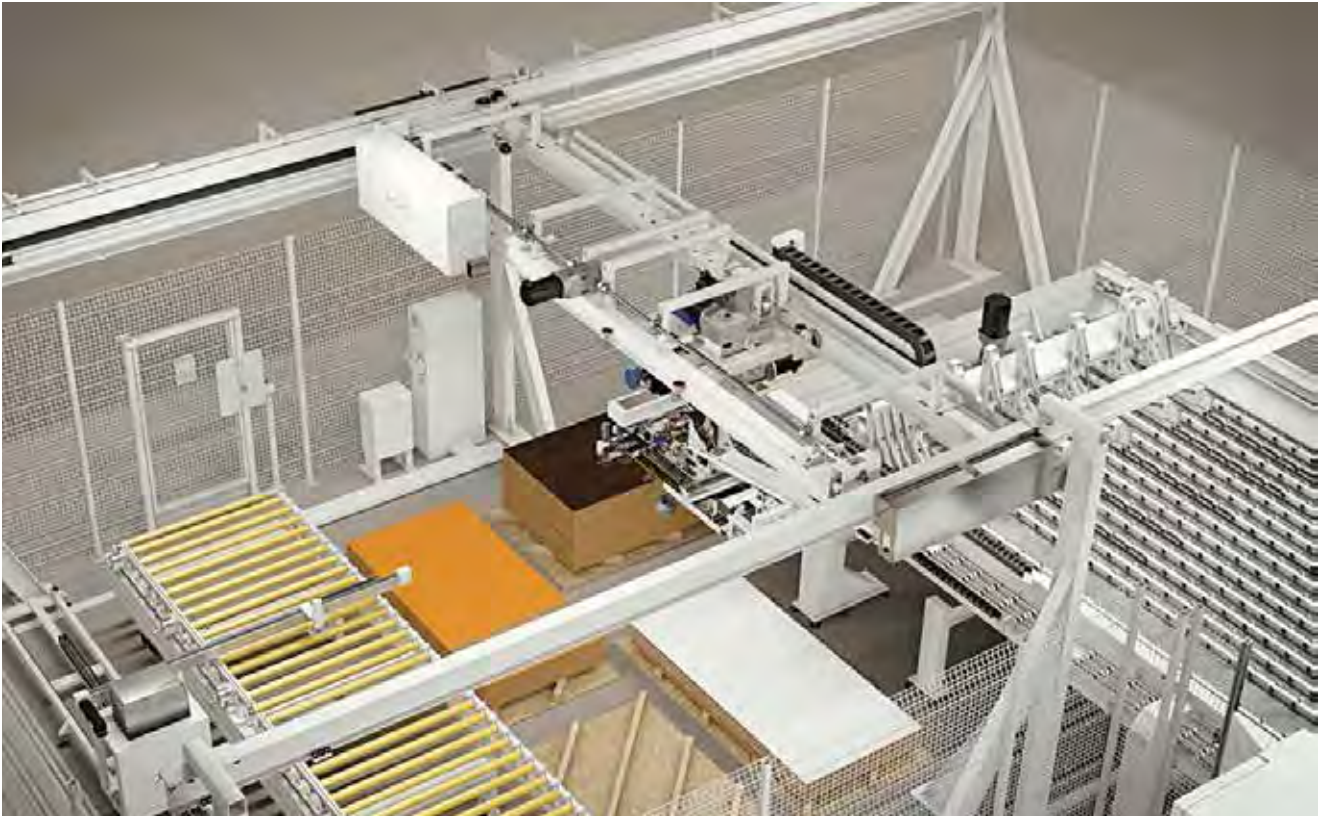
Secure and precise panel transfer. The suction cup arm automatically adapts to the different lengths and widths of the panels to be picked up.
