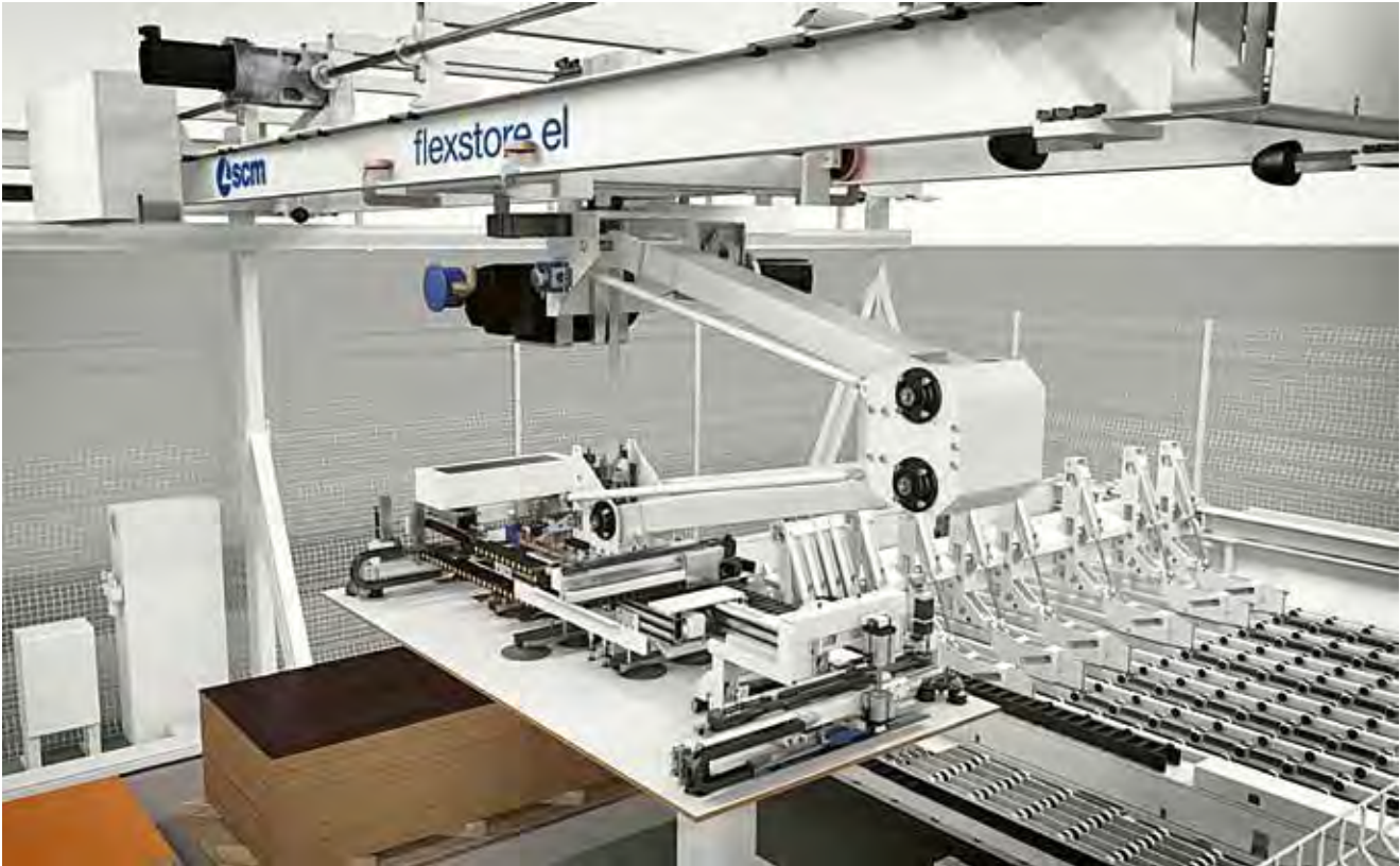
Secure and precise panel transfer. The suction cup arm automatically adapts to the different lengths and widths of the panels to be picked up.
