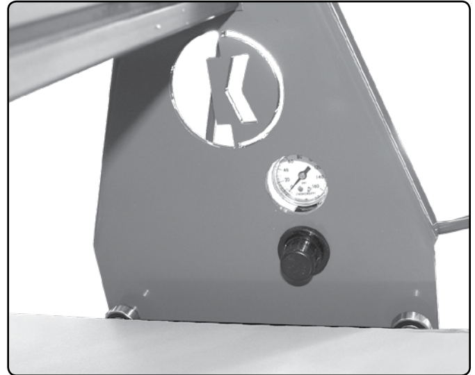
Regulator controls amount of air pressure to the screw gun.
