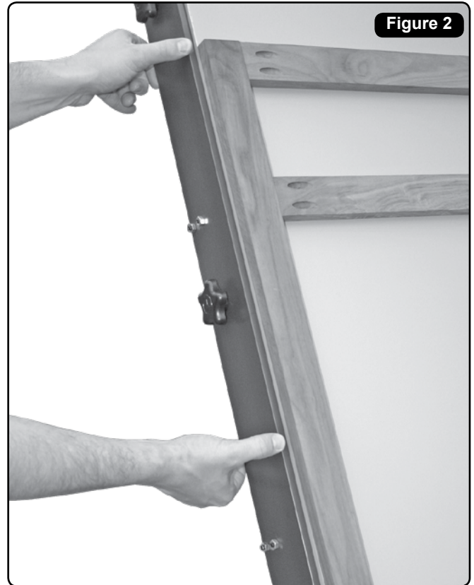
Lift fence up and down to move out of the way
