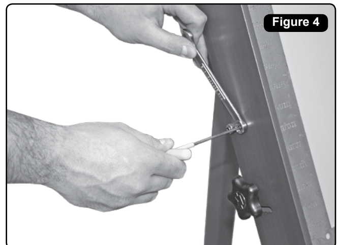
Re-tighten locking nut once complete.
