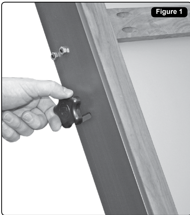
Loosen locking knobs on side of fence
