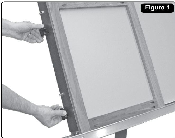
Place workpiece into alignment with squaring fence
