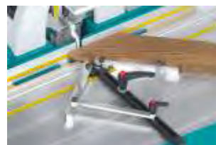
Adjustable fence "Synchro" 0-90°
