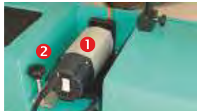
Machine components 1. Router motor 2. Height adjustment
