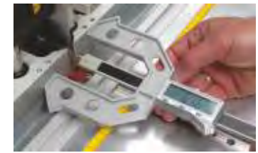
Digital Multi Gauge for accurately setting of router bits (W 2001300)
