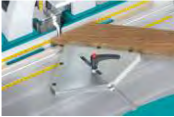
45 degree Center Fence Plate for joining 4-sided frames (W3060001)
