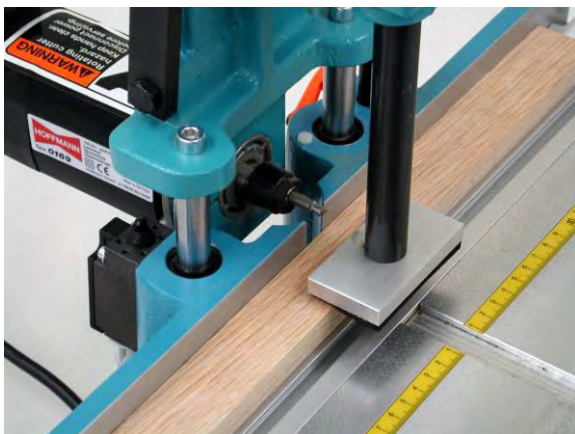
Scrap wood for initial cut though new chip breaker
