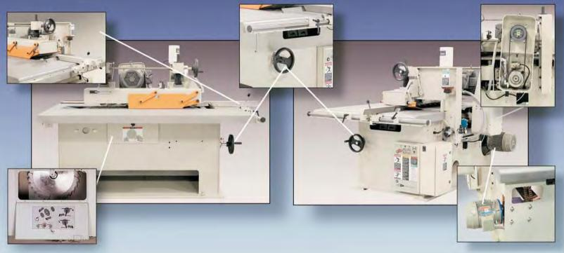
The front view illustrates access into the electrically interlocked saw pit area, the dual anti-kickback finger system, pivoting pressure beam side guard and the standard rail mounted stock guide.
