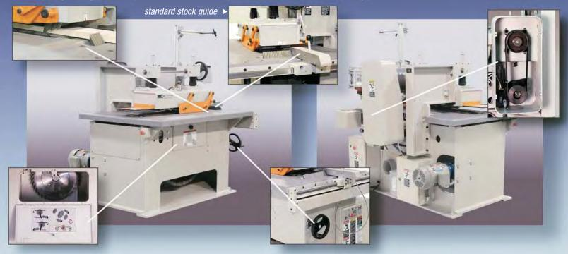
The front view illustrates access into the electrically interlocked saw pit area, the dual anti-kickback finger, system the pivoting pressure beam side guard and the adjustment handwheel to accommodate correct positioning of the saw blade for varying thicknesses of material.
